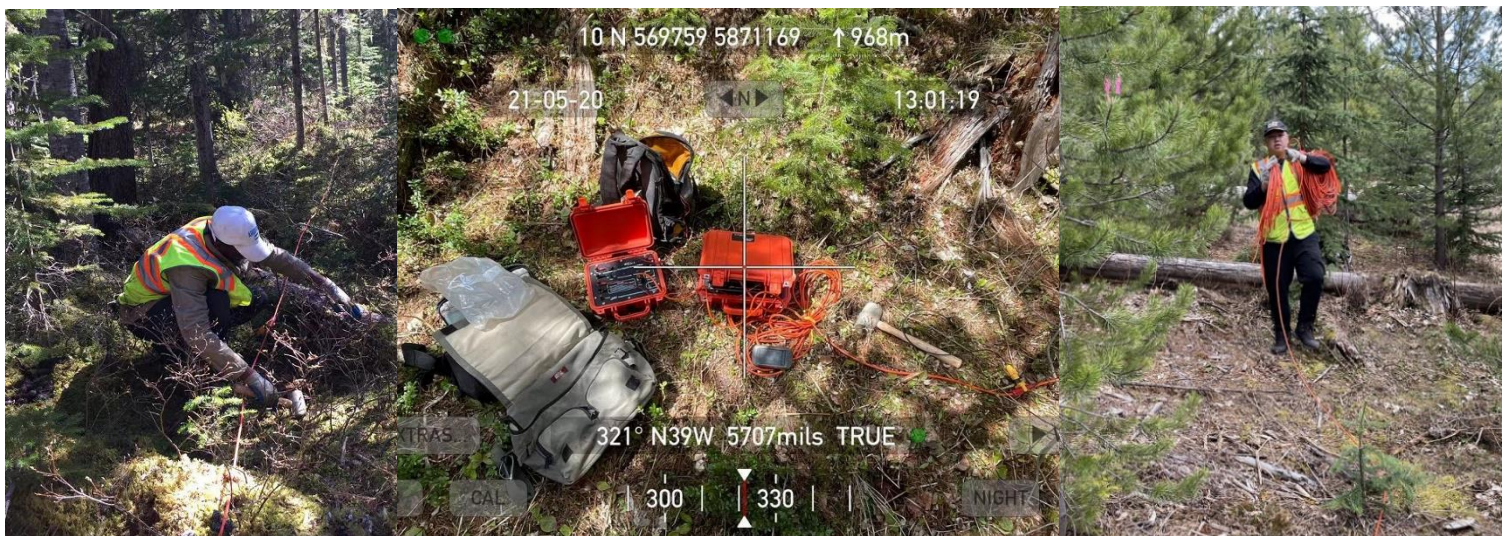
Figure 7 Working Photos. The geophysical technicians were performing the 2D Resistivity Survey, in Cariboo Regional District, BC. Fargo Exploration Ltd., 2021.
