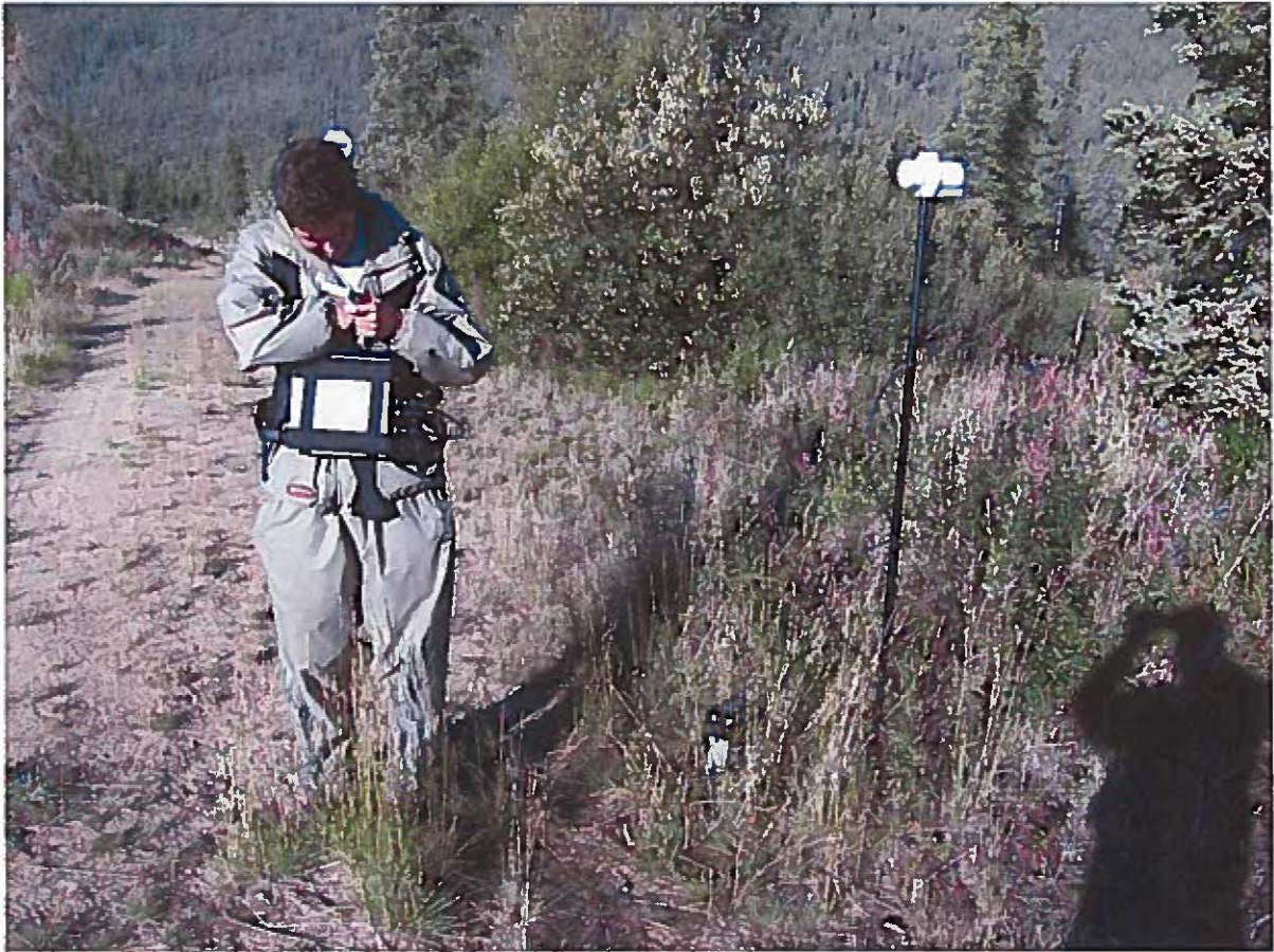
Magnetometer Survey – Dolly Creek – photo taken August 2017 --The rover magnetometer is strapped to the operator's chest and the sensor coil is above his head.
