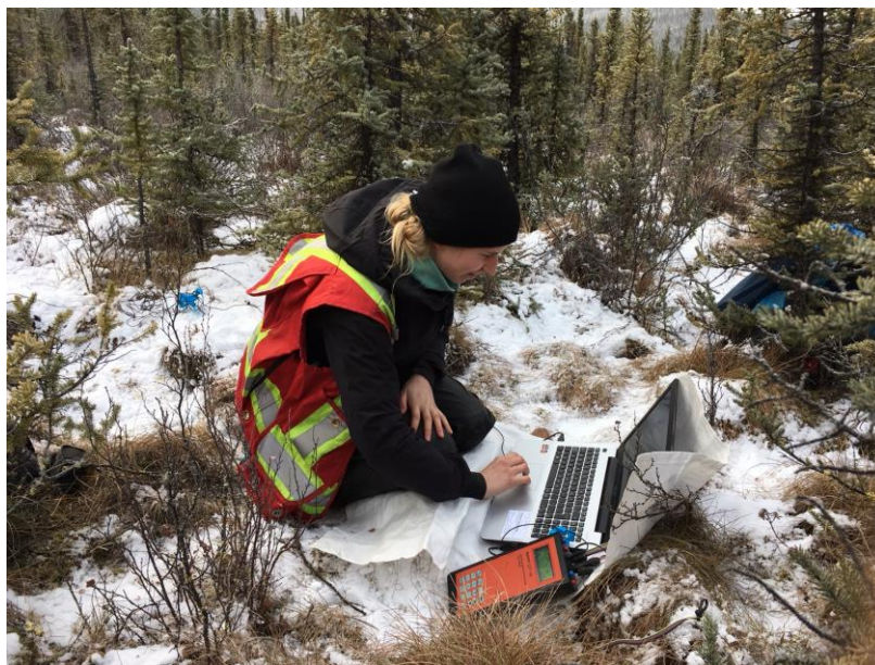
Photo 1: Setup including Lippmann 4 Point Light resistivity meter and field laptop.
