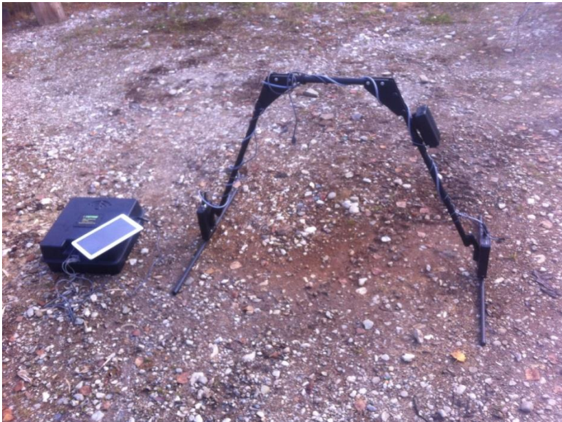
The two georadars used at Simmons Creek: “Scudo 500” (left) and “Dipole 300” (right)
