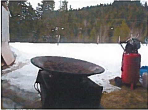
Hotplate used for drying
