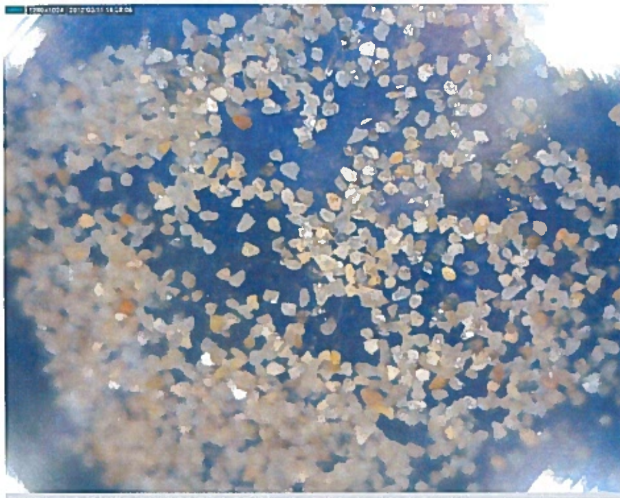
Overflow of rising current classifier 40-70 test
