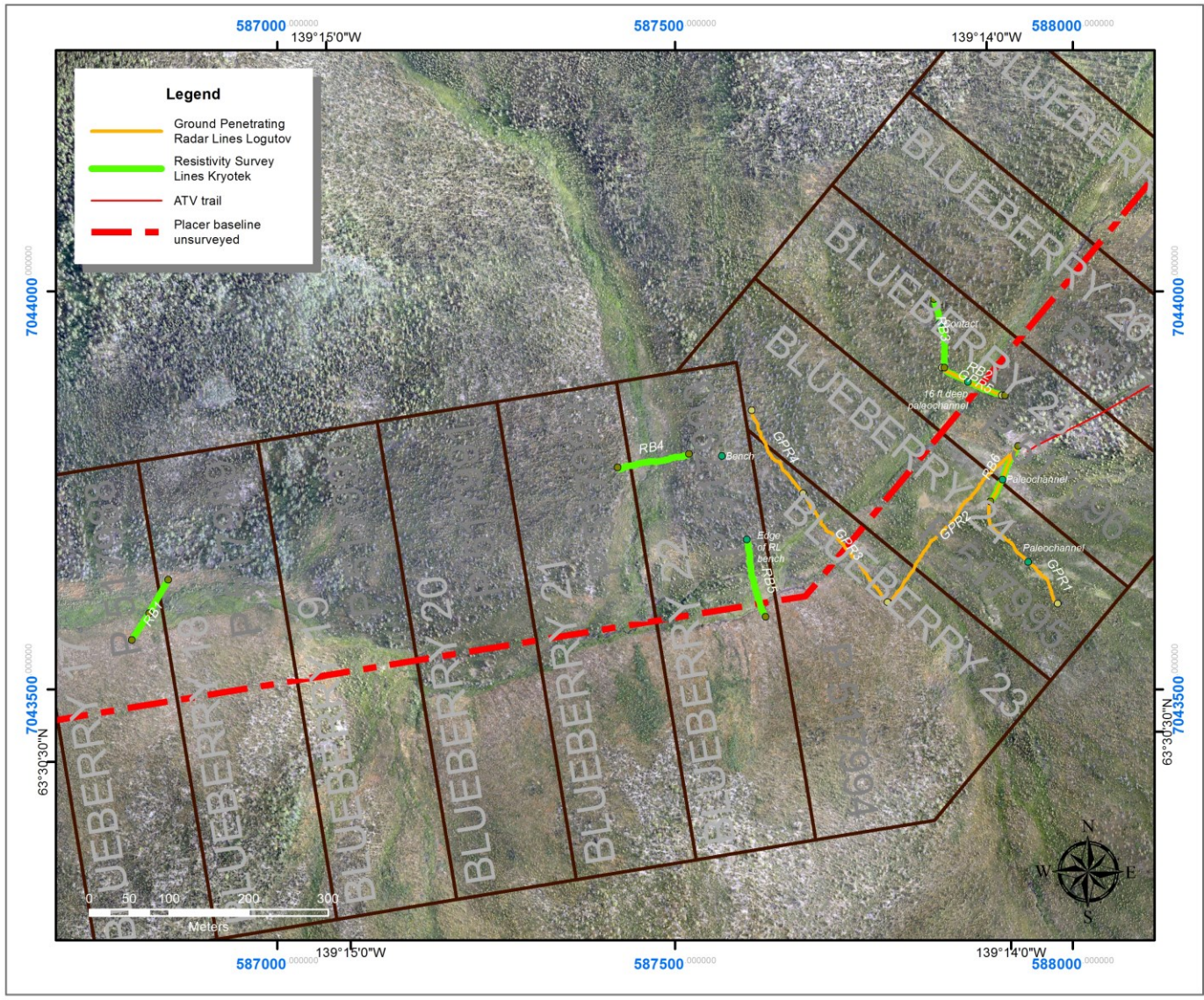
Figure 14 - Location of the 2016 Kryotek resistivity survey lines and the Logutov ground penetrating radar survey lines on upper Rosebute Creek.
