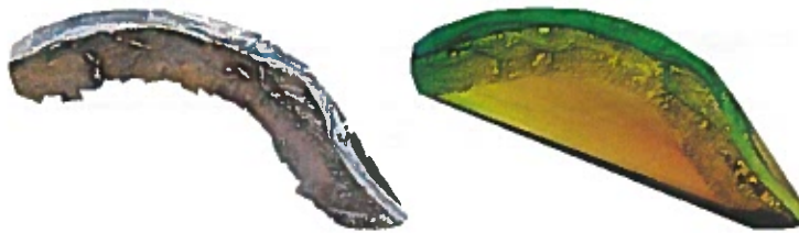
Figure 1: Orthomosaic and the corresponding sparse Digital Surface Model (DSM) before classification.
