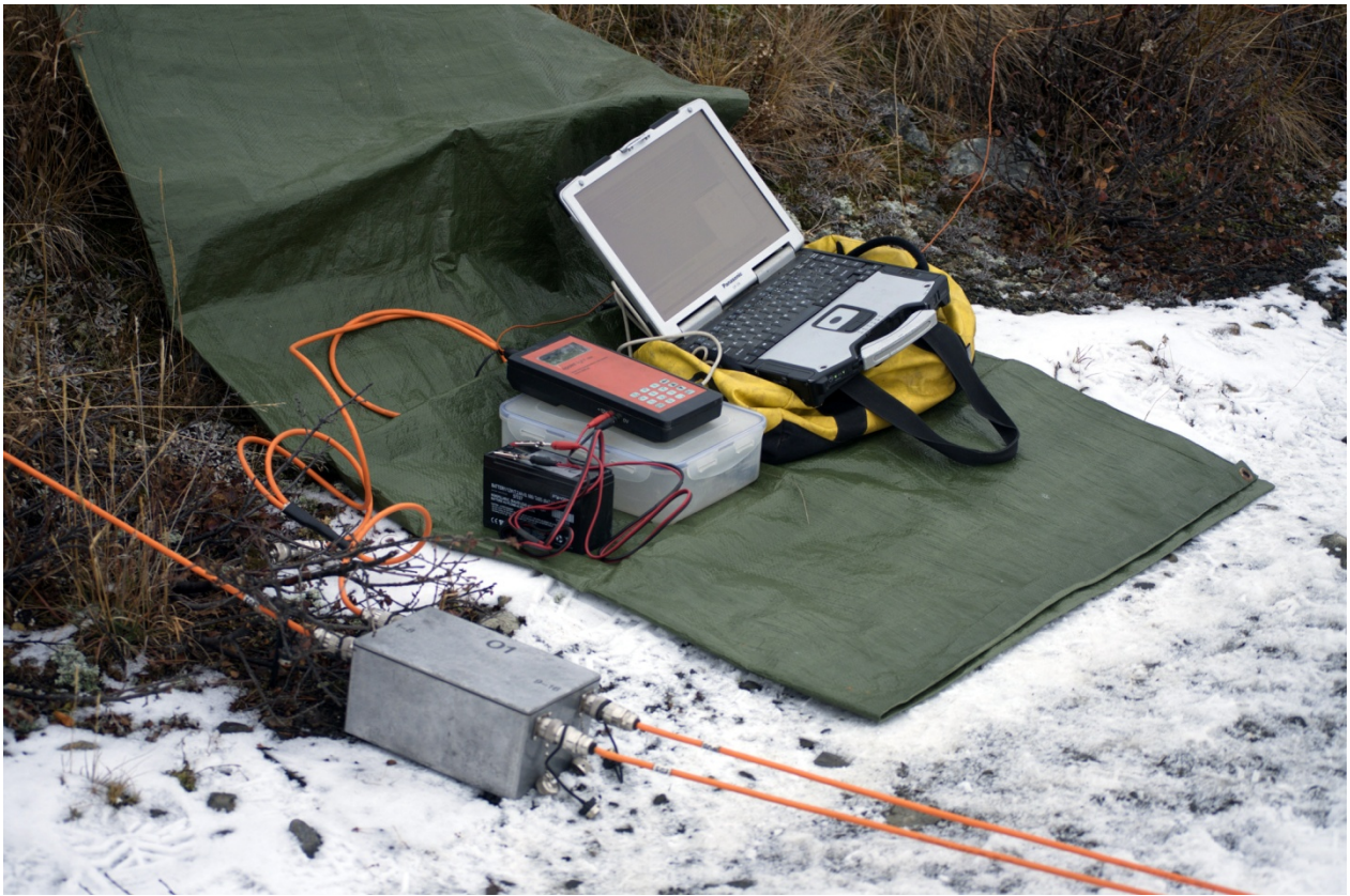
Figure 1: 2D Resistivity/IP measurement, Stefan Ostermaier, Arctic Geophysics Inc., Atlin, BC 2013
