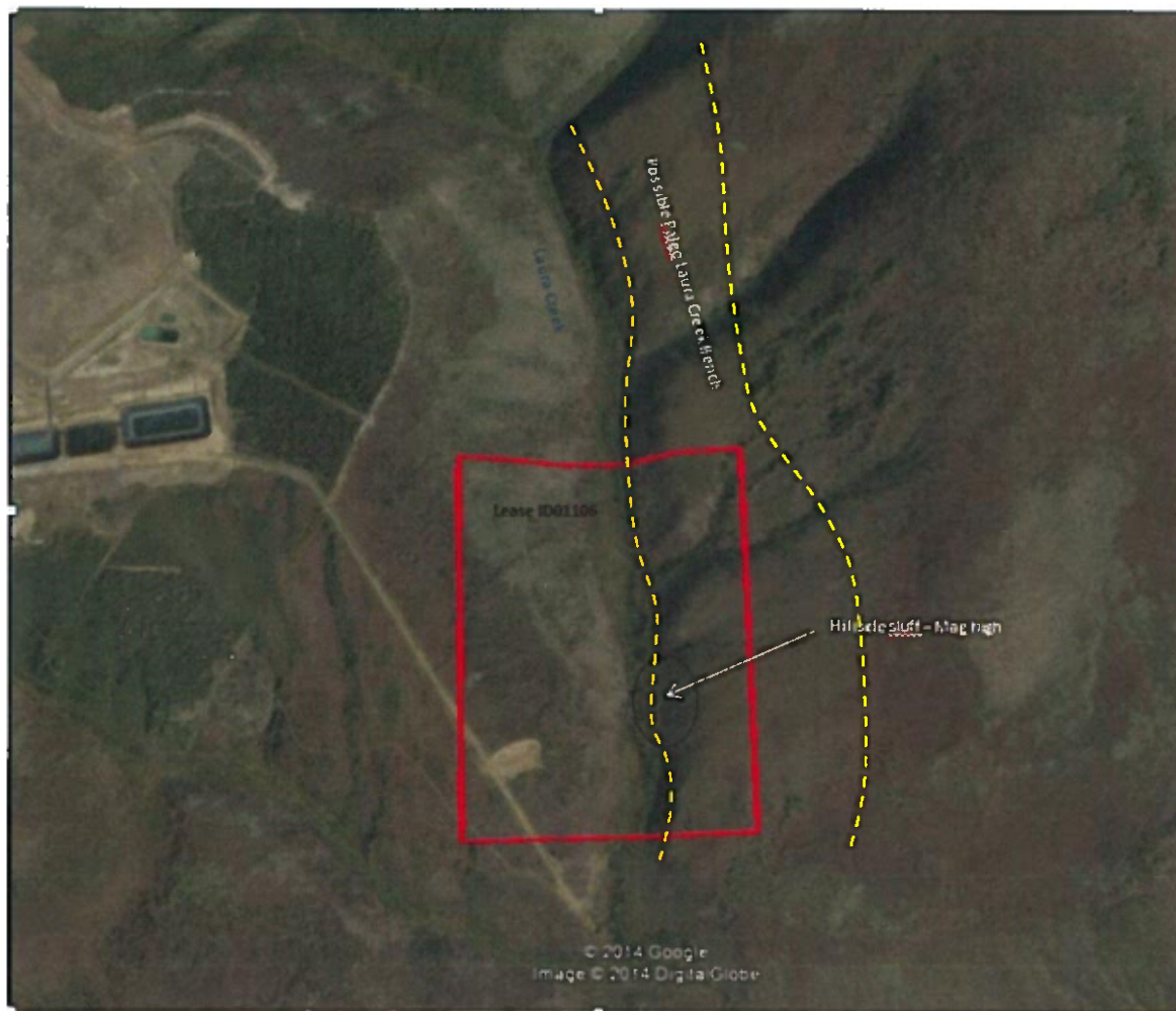
FIGURE 6: AIR PHOTO shows lease ID01106 projected on google earth. Note: the yellow dotted lines show the inferred paleo bench and the black circle highlights a sluff of the bench that was recorded as a magnetic high in the survey.
