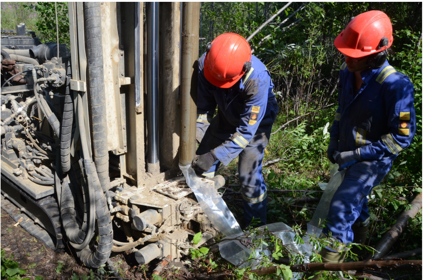
Plate 4 - Sonic drill core was recovered into plastic sleeves and put into core boxes for logging.
