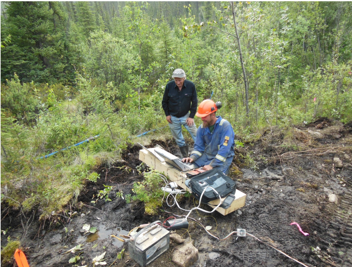
Plate 3- Resistivity results were plotted in real time in the field to aid in drillhole targeting.
