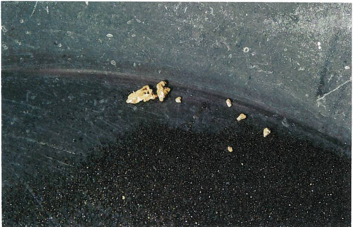
Photo 7: Sample 5 (Left Limit Trench) showing course-hackly gold nuggets and black heavy mineral concentrate in metal gold pan.
