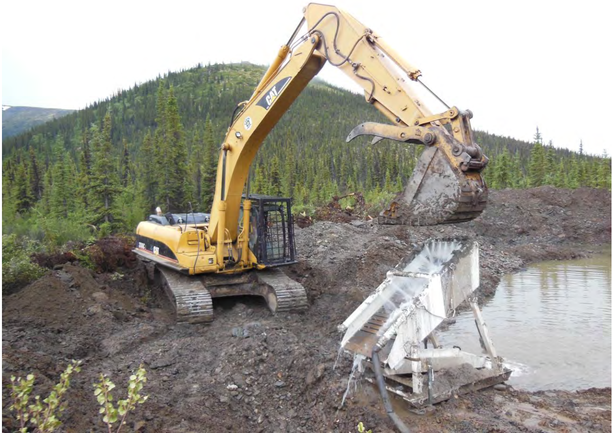
Figure 24 - The field test plant was fed directly by an excavator.
