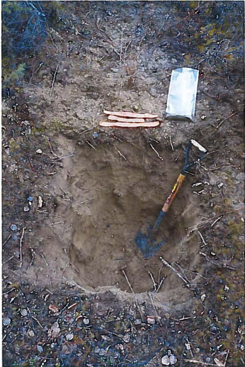
Plate 4 - Test Pit Max #2 encountered a sand layer with gravel at the bottom.
