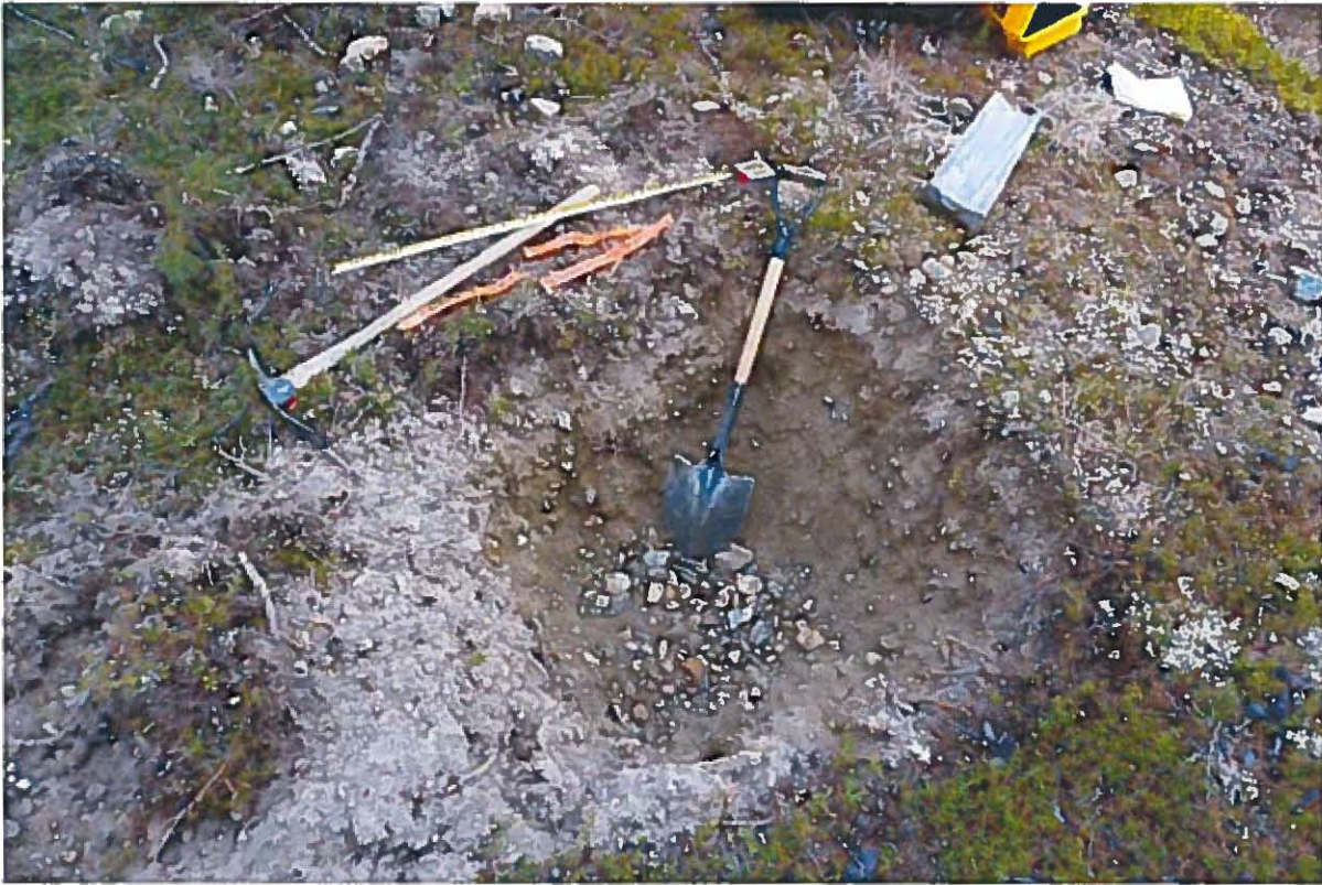
Plate 6 - Test Pit Max #4 encountered a sandy gravel under a thin layer of moss.
