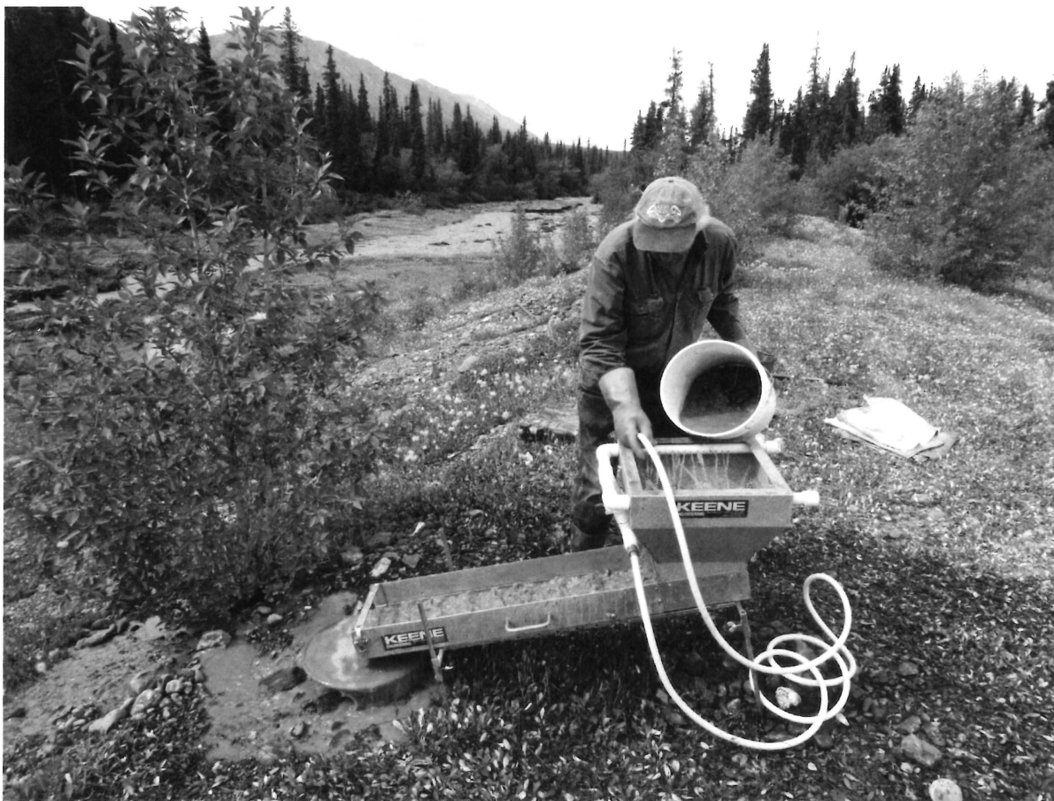
Plate 3 - Drill samples were processed in the field using a Keene A52 sluicebox.
