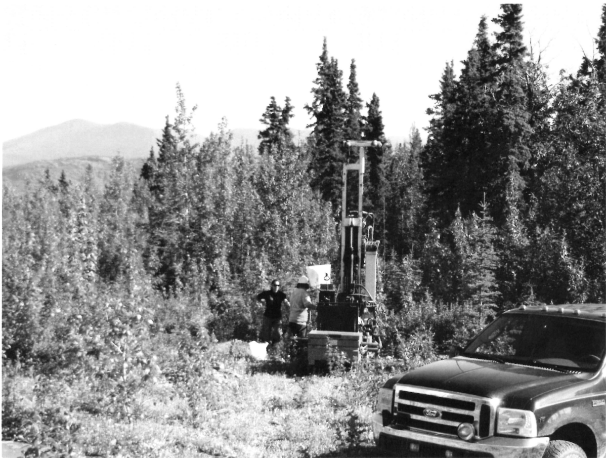
Plate 2 - Sonic drill collaring a drill hole in the lower claim area.
