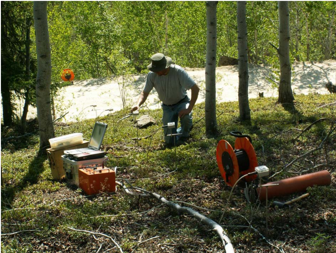
Figure 5: 2D Resistivity/IP measurement, Stefan Ostermaier, Arctic Geophysics Inc., Yukon 2009 (Moll)
