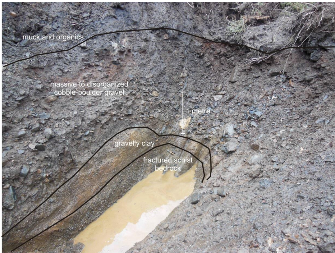
Plate 7 - Excavator test-pit CAN14-01, showing the stratigraphy down to bedrock. View looking south-southwest.
