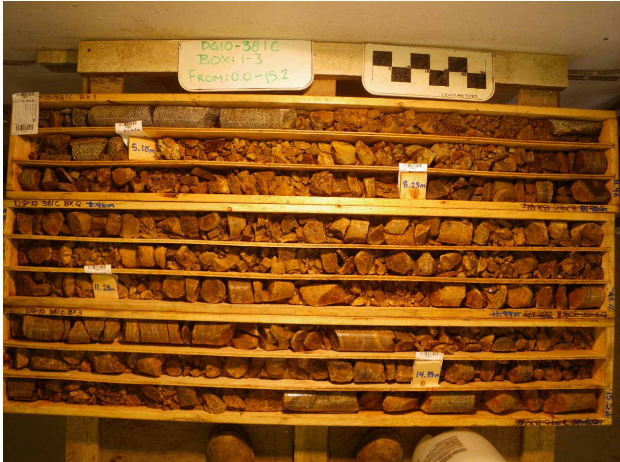
Picture 1: Wet photo of logged core from the top of hole DG10-381C.
