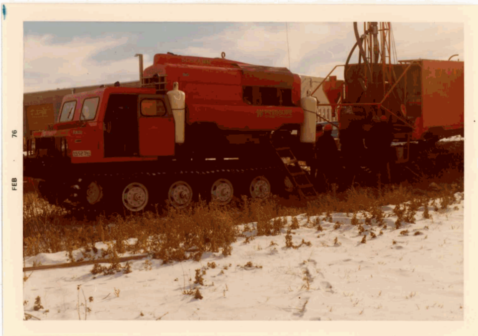
Plate II : The Nodwell RN 110 which carries the compressor. Here it is shown hooked up to the drill ready to work. The drill unit is shown to the right of the picture.
