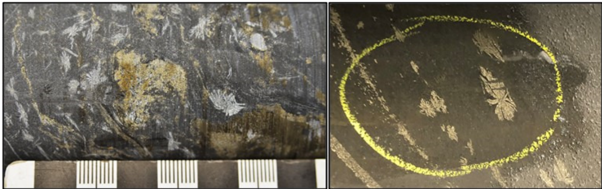
Figure 7.4.1. Radial splays of barite needles (“snowflakes”), partially to completely replaced by pyrite.
