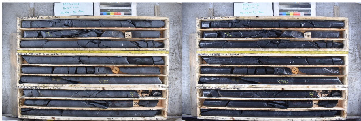
Figure 8.3. Core photos from MP20-001 showing massive, black, carbonaceous mudstone (dry/wet).
