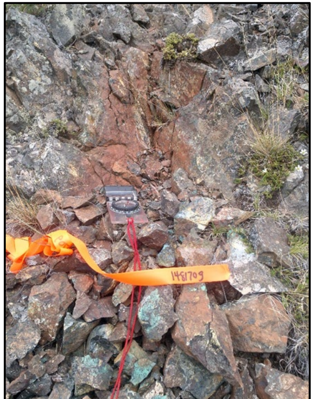
Figure 6-5: Andesite porphyry from Zone D with malachite and hematite staining. Sample 148709 ran 0.74% Cu and 0.406 g/t Au
