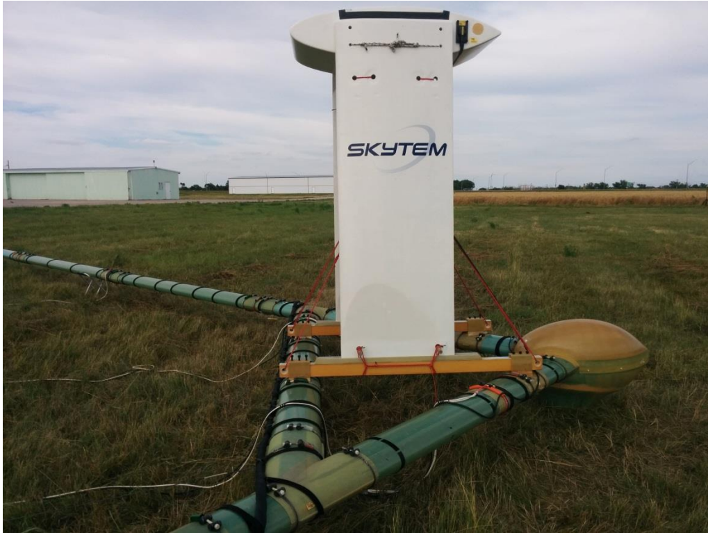
Figure 22 Rudder containing the Z coil located in the top part of the tower.
