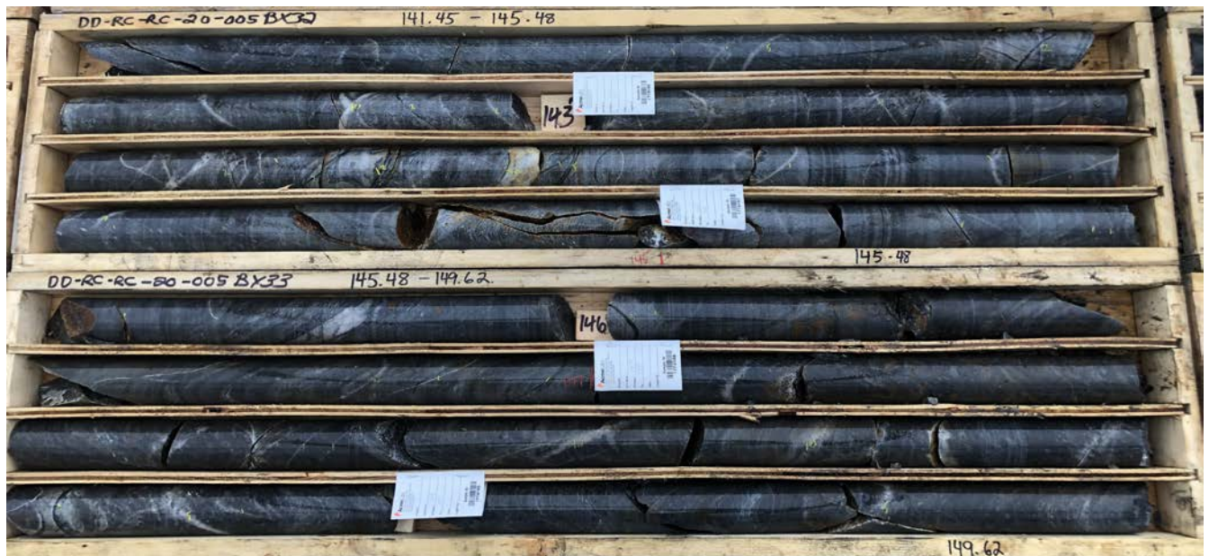
Figure 11 - Typical section of hornfelsed metasediments with qtz veins from hole 5 (141.45-149.62m)
