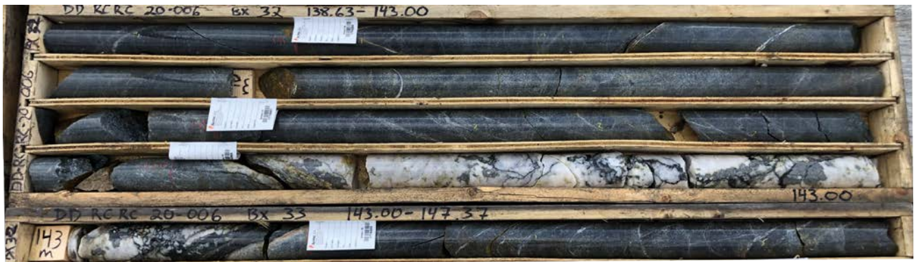
Figure 12 - 1.2 meter intersection of Qtz-Tourmaline-Arsenopyrite vein from hole -006
