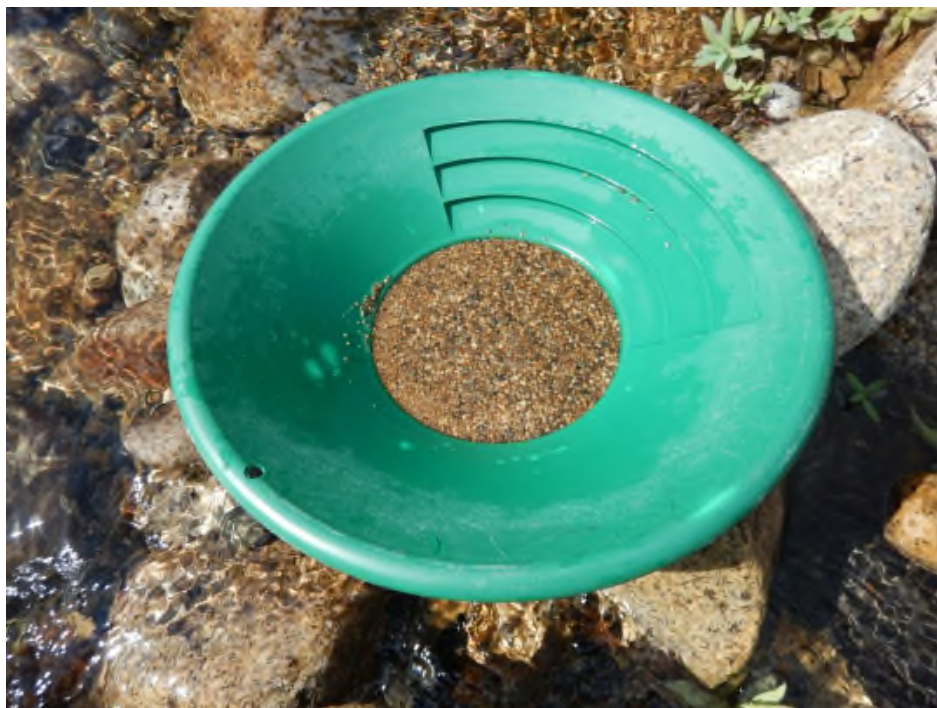
Figure 12. Photo showing stream sediment heavy mineral concentrate sample after concentration by panning (heavy mineral concentrate sample SR701; 376236E, 6665434N, UTM NAD83 Zone 9V).
