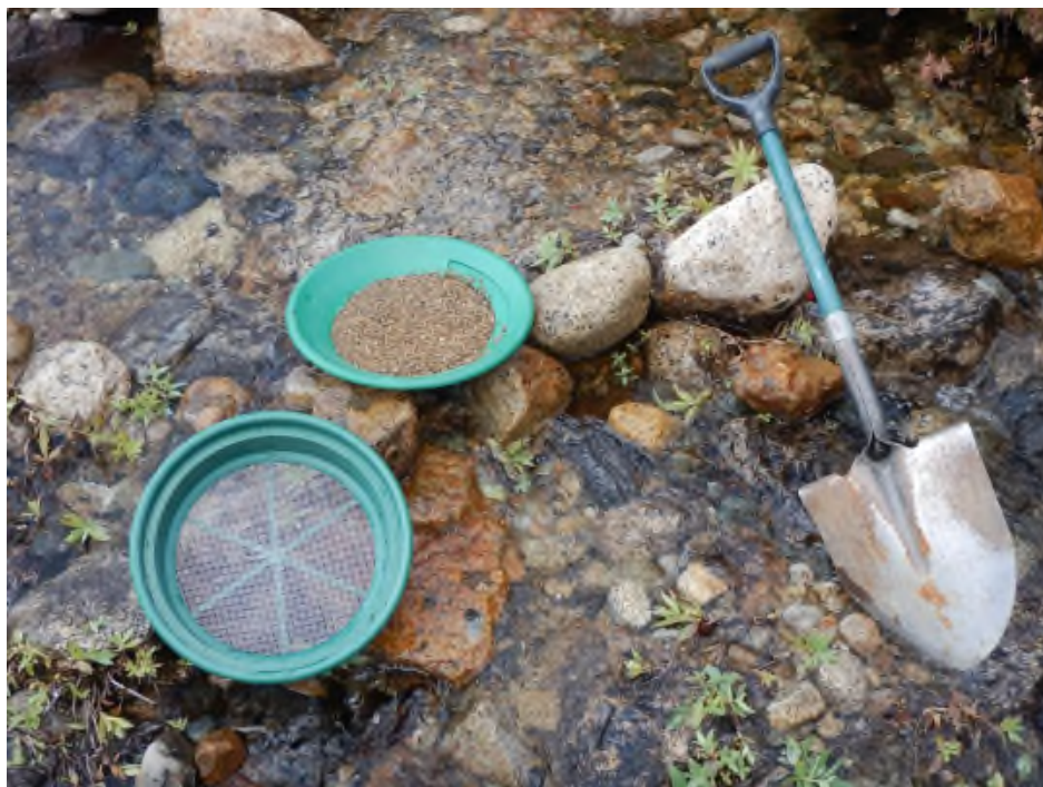
Figure 11. Photo showing stream sediment in pan after sieving and before concentration by panning (heavy mineral concentrate sample SR701; 376236E, 6665434N, UTM NAD83 Zone 9V).
