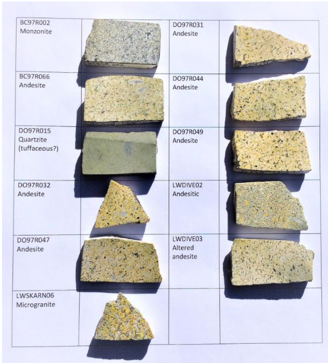
Figure 11 Historical Thin Sections (1997) - Potassium Staining
