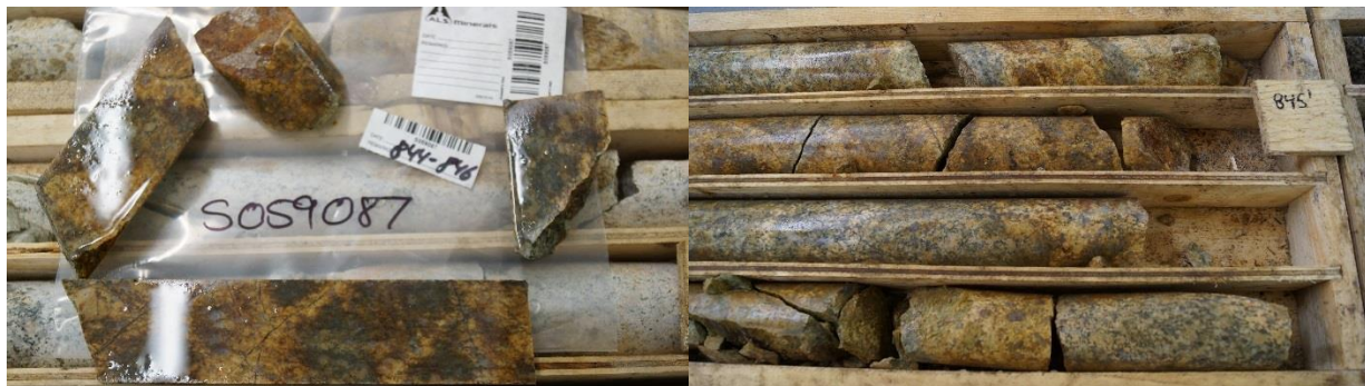
Image 2. Pervasive chloritization with jasper-quartz veinlets.
