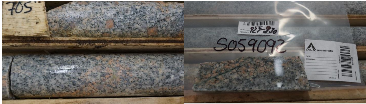
Image 1. Potassic alteration in core, locally with partially replaced plagioclase grains
