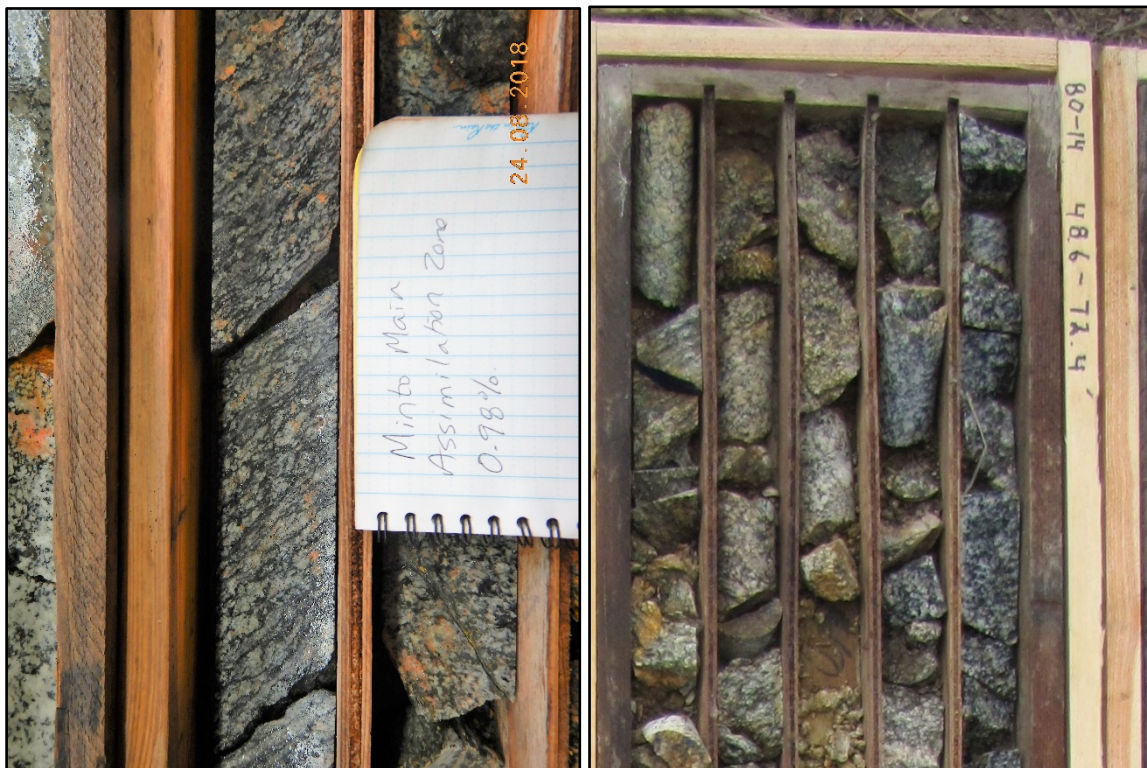
Figure 7.5: Example of assimilation zone in Minto core on left and in Stu core on right. Note the foliation defined by segregation of felsic and mafic minerals. Photo on left by author, photo on right by YGS.
