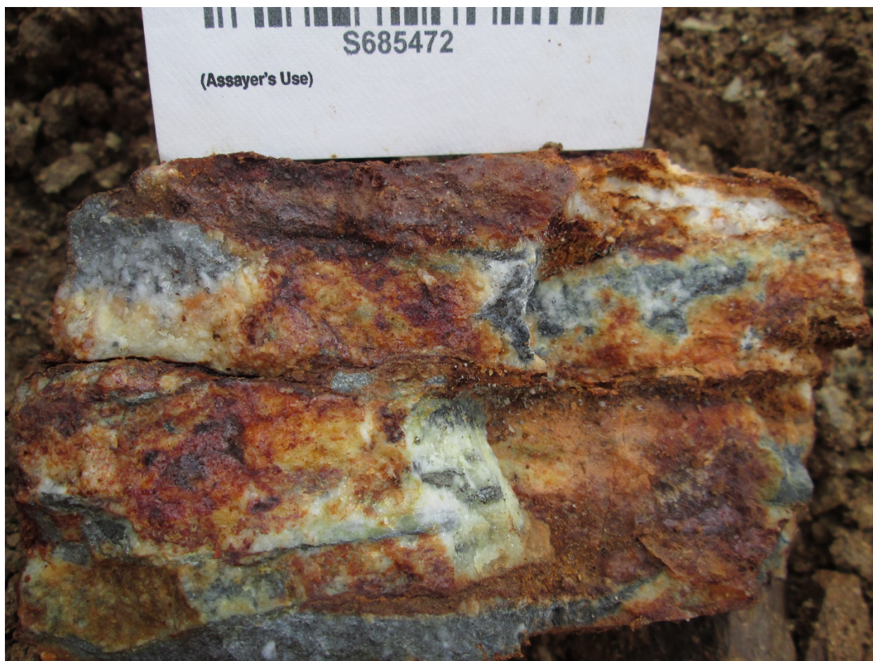
Photo 3, Quartz vein float with disseminated stibnite and arsenopyrite (arsenia pyrite) bands and pods returns 9.93 g/t Au, 2.89 g/t Ag, more than 10000 ppm As and Sb.
