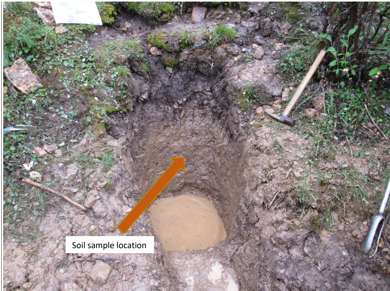
Photo 4, High Grade zone shallow pit digging, 1.2 meters depth, loose materials with quartz chips. Soil sample returns 5.31 g/t Au. (No bad rock explored)
