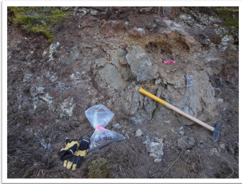
PHOTO 2. POND ZONE, ROCK SAMPLE Q009322 (373 PPB AU) FROM STRIPPED OUTCROP AND SOIL SAMPLE I030102 (42.1 PPB AU) AT PINK RIBBON, HAMMER IS APPROXIMATELY 75 CM LONG.
