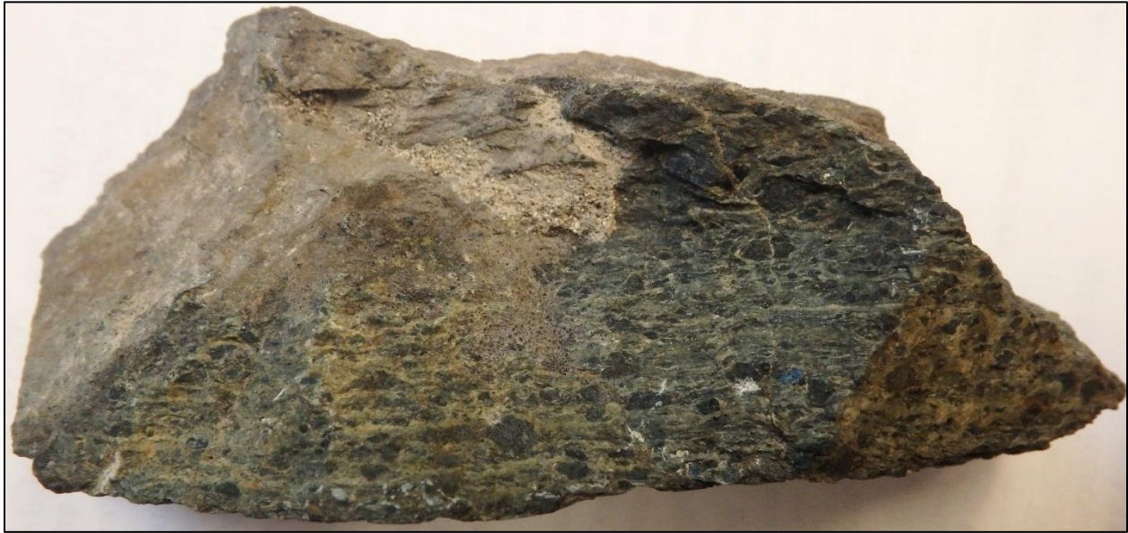
Figure 4 Weakly foliated augite phyric basalt, tentatively correlated with the Povoas formation, Lewes River Group. Left to right field of view is 11 cm. Sample taken from the WASP 48 claim at NAD83 UTM Z8N (412,215 – 6,921,567).
