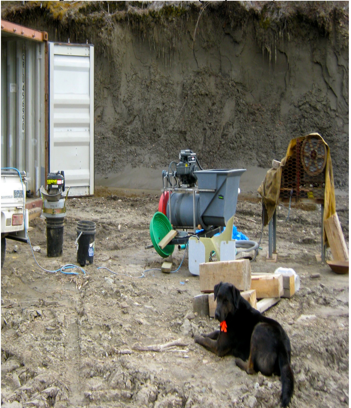
Crushing and pulverization equipment utilized to recover specimens pictured from CripPit. (Some assaying will not capture “visible” gold unless special request is made for large mesh). This method helps to target sample zones in a more economic and reliable way while prospecting.
