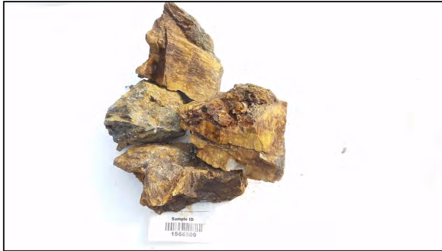
Figure 8: Sample 1566509 (43.4 g/t Au); Qz-As veinlets in phyllite
