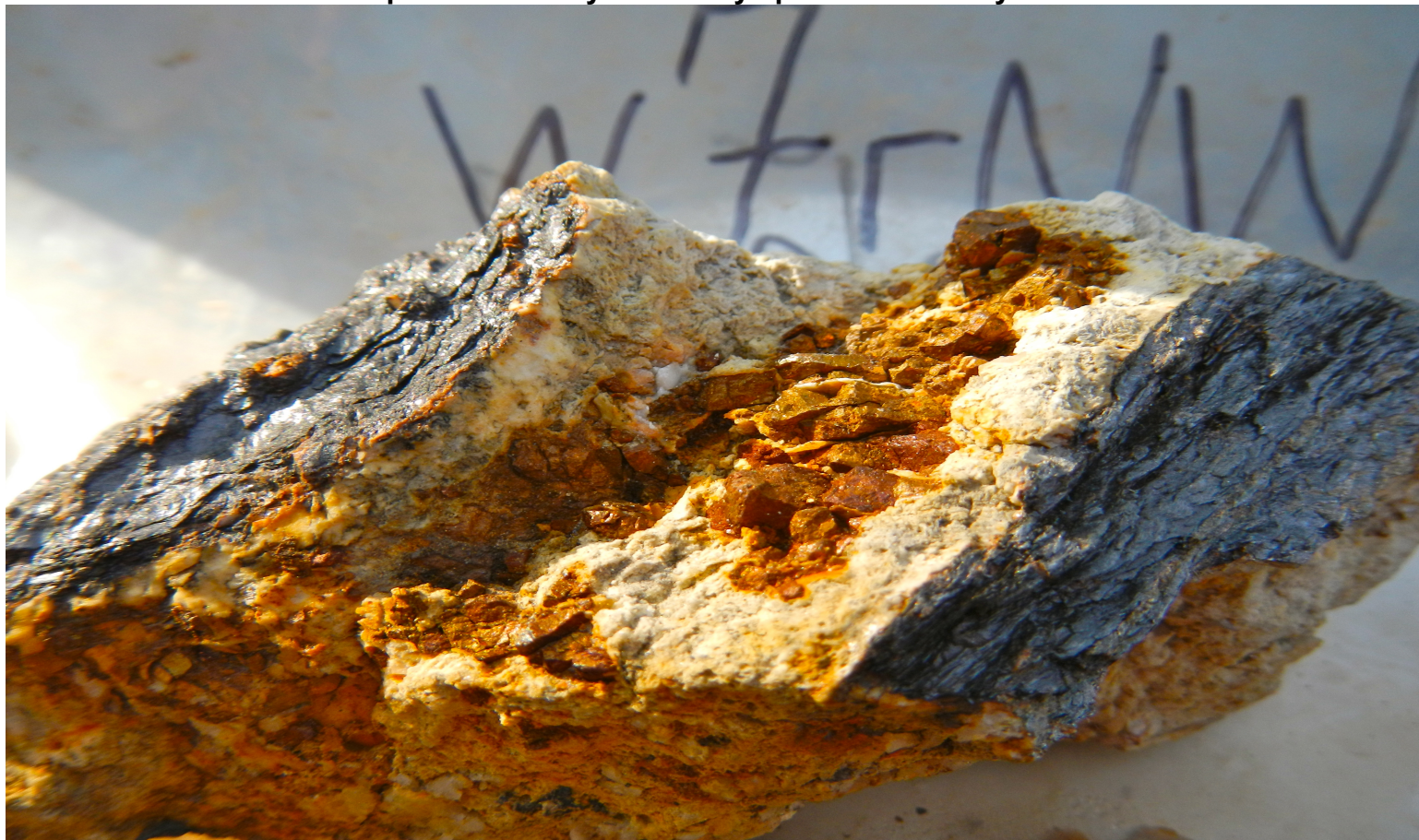
w7rNw – 2013, assayed 581gm/ton Arsenic, 461gm/ton Cobalt, 340gm/ton Nickel, 23gm/ton Silver & 5.71gm/tonAu.
