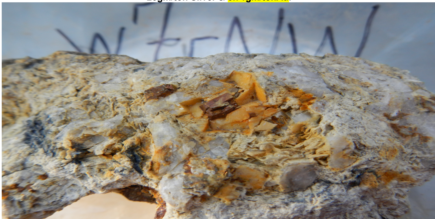
w7rNw – 2013, assayed 581gm/ton Arsenic, 461gm/ton Cobalt, 340gm/ton Nickel, 23gm/ton Silver & 5.71gm/tonAu.
