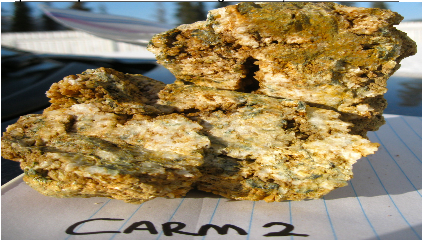
Carm2 – Hydrothermally altered sericite/chlorite schist coated quartz/feldspar lenses and veins. Orange oxidation, small sulfides visible.
