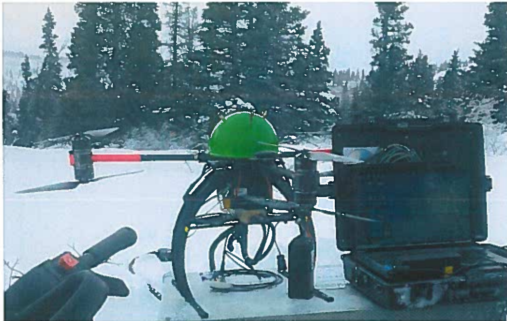
Figure 3 Pioneer Exploration's UAV-MAG™ system.
