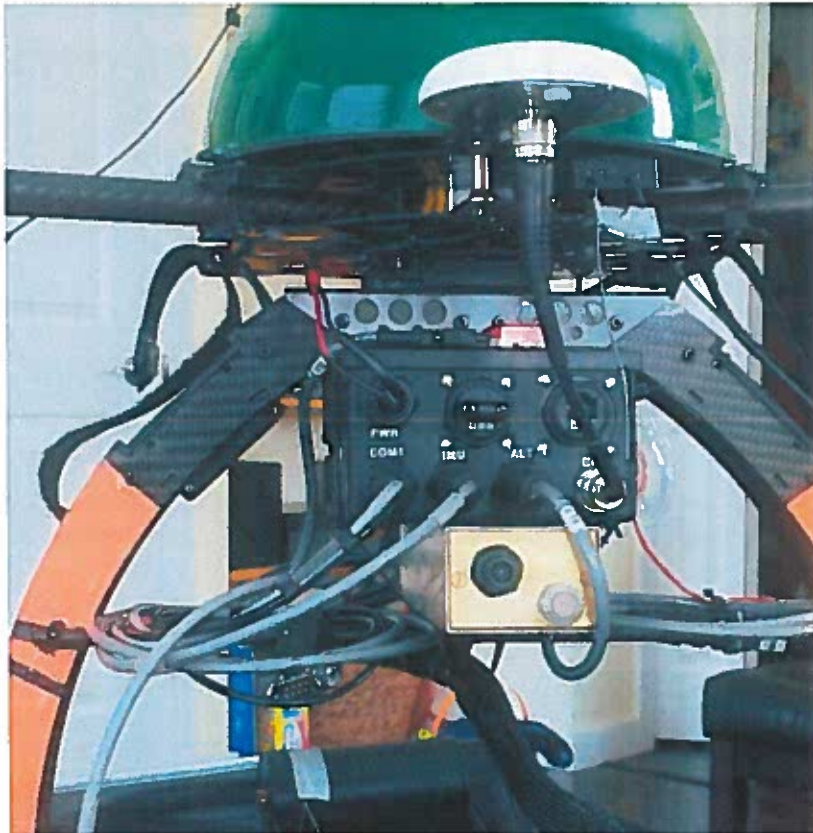
Figure 4 Airborne instrument rack.
