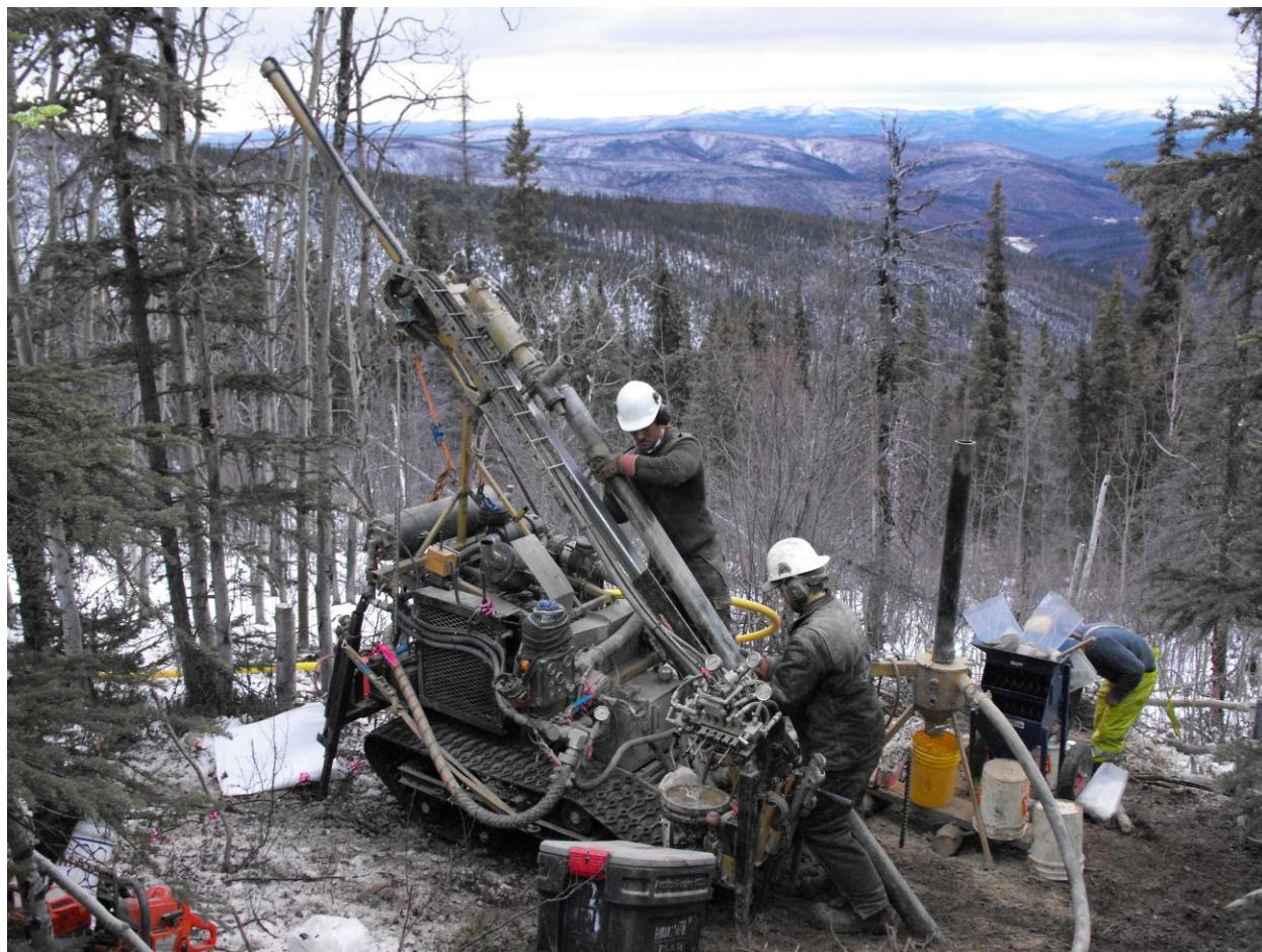
Figure 9: Ground Truth's track mounted RAB drill.
