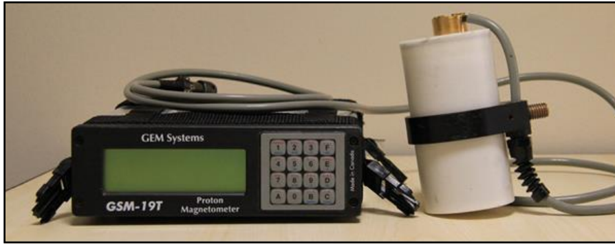
Figure 14: GEM GSM-19T proton precession magnetometer.
