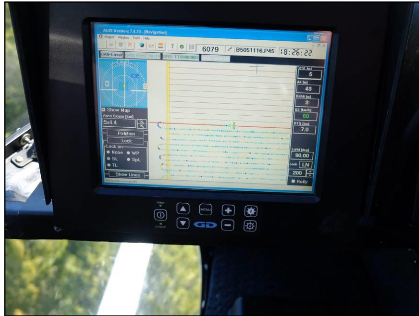
Figure 11: AGIS operator display installed in the Eurocopter AS350, with screen displaying real time flight line recording and navigation parameters. Additional windows display real time geophysical data to operator
