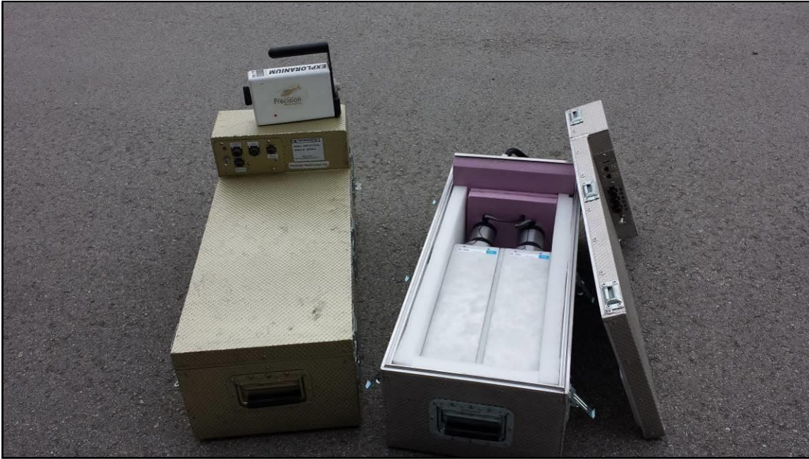
Figure 13: GRS-10 Thallium-activated Sodium Iodide spectrometer crystal pack. The open unit on the right shows two individual 4.2 liter detectors.
