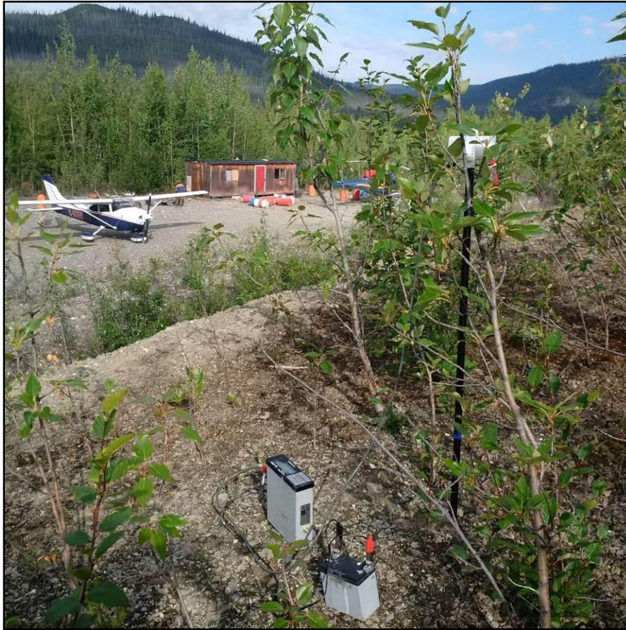
Figure 7: GEM 3 (right) magnetic base station at Russell Creek airstrip.
