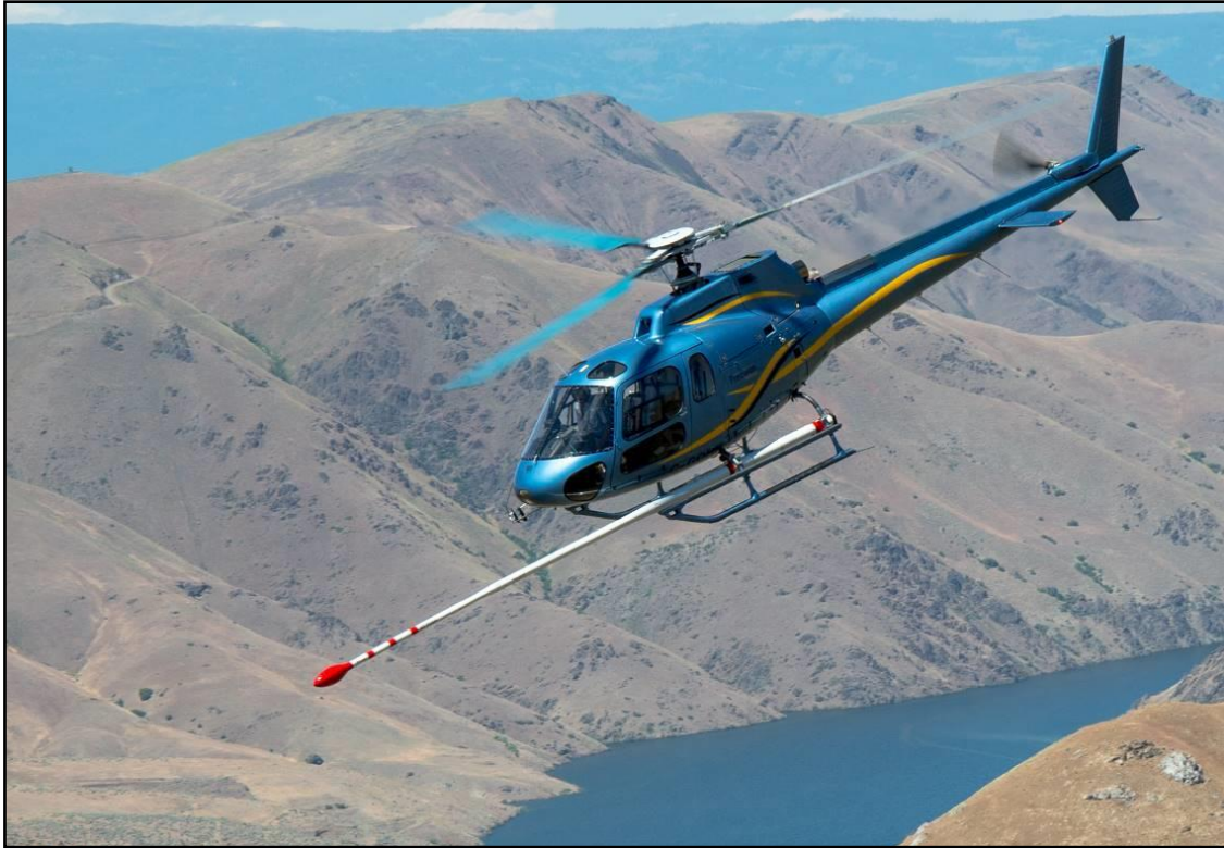
Figure 10: Eurocopter AS350 helicopter equipped with mag stinger for magnetic data acquisition, and internal spectrometer crystals for radiometric data acquisition.
