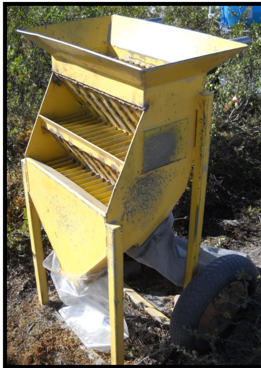
Figure 8 Splitter used to obtain 2-5 kg representative sample.
