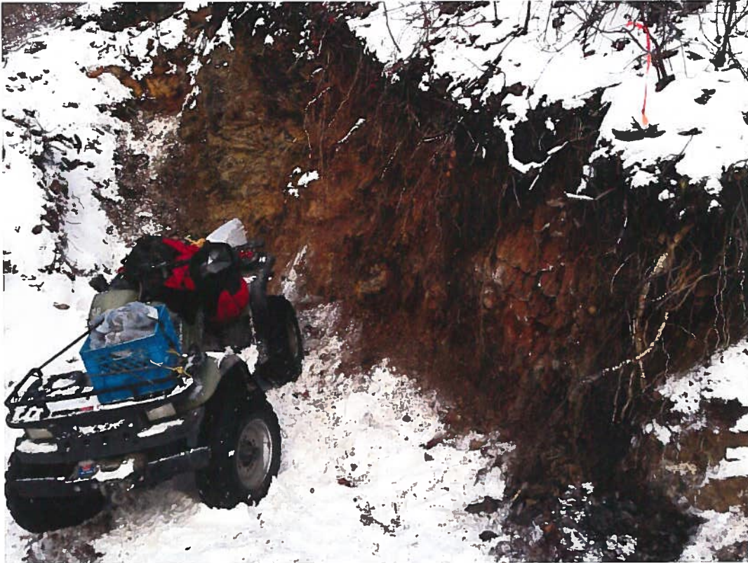
Sampling Hwy Fault Zone. Trench cuts across fault zone with listwanite breccia at top grading to sheared argillite at bottom.
