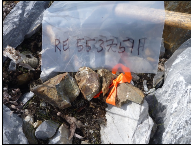
Figure 7: Sample RE5537511: Trench push, arsenic veining in felsic dyke returning 23.54 g/t gold
