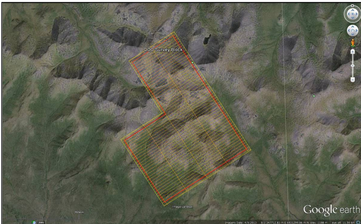
Figure 3: Plan View – OOO survey block with actual survey and tie lines displayed in orange, the 100 m buffer zone outline in yellow, and the block boundary in red.
