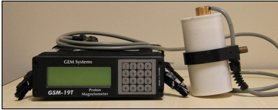
Figure 19: GEM GSM-19T proton precession magnetometer.
