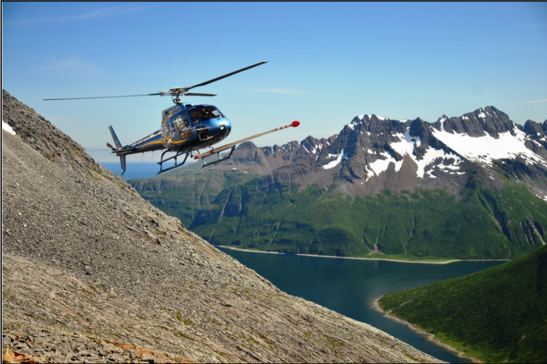
Figure 15: Eurocopter AS350 helicopter equipped with mag stinger for magnetic data acquisition, and internal spectrometer crystals for radiometric data acquisition.
