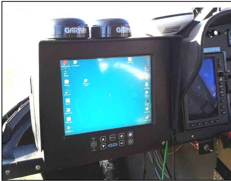
Figure 16: AGIS operator display installed in the Eurocopter AS350.
