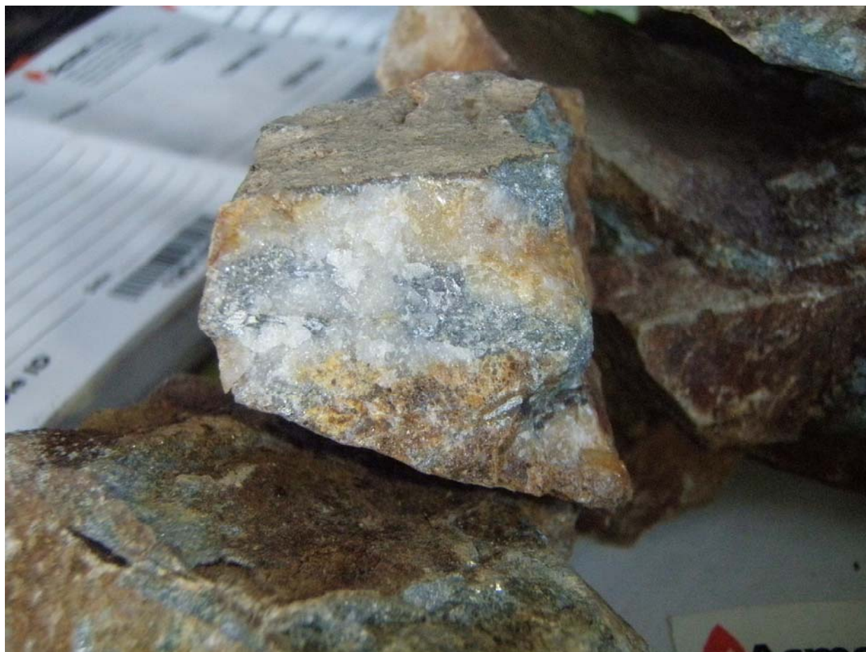
Photo 2: Sample 1201915 assayed 4390 ppb Au, <10000 ppm As, 182 ppm Pb, 159 ppm Co, 434 ppm Sb, 69 ppm Bi, and 3.7 ppm Te.
