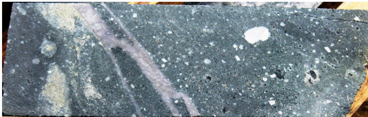
Figure 14: Plagioclase-phyric porphyry with pervasive chlorite alteration and disseminated pyrite-(chalcopyrite-molybdenite). The porphyry is cut by an aplite vein with disseminated chalcopyrite and molybdenite.
