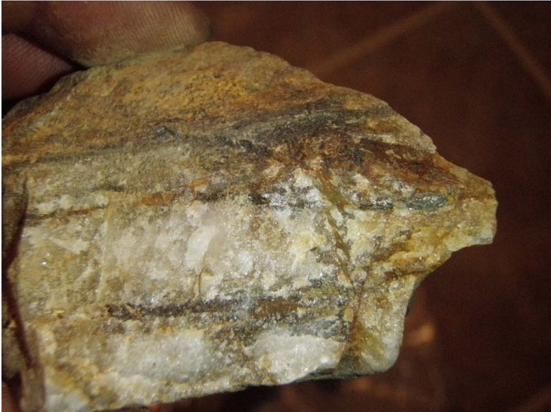
Photo 2: Rock sample 1201911 yielded 44.3 ppb Au, 3100 ppm As, 984 ppm Pb, 128 ppm Zn, 602 ppm Mn, and 473 ppm Sb.
