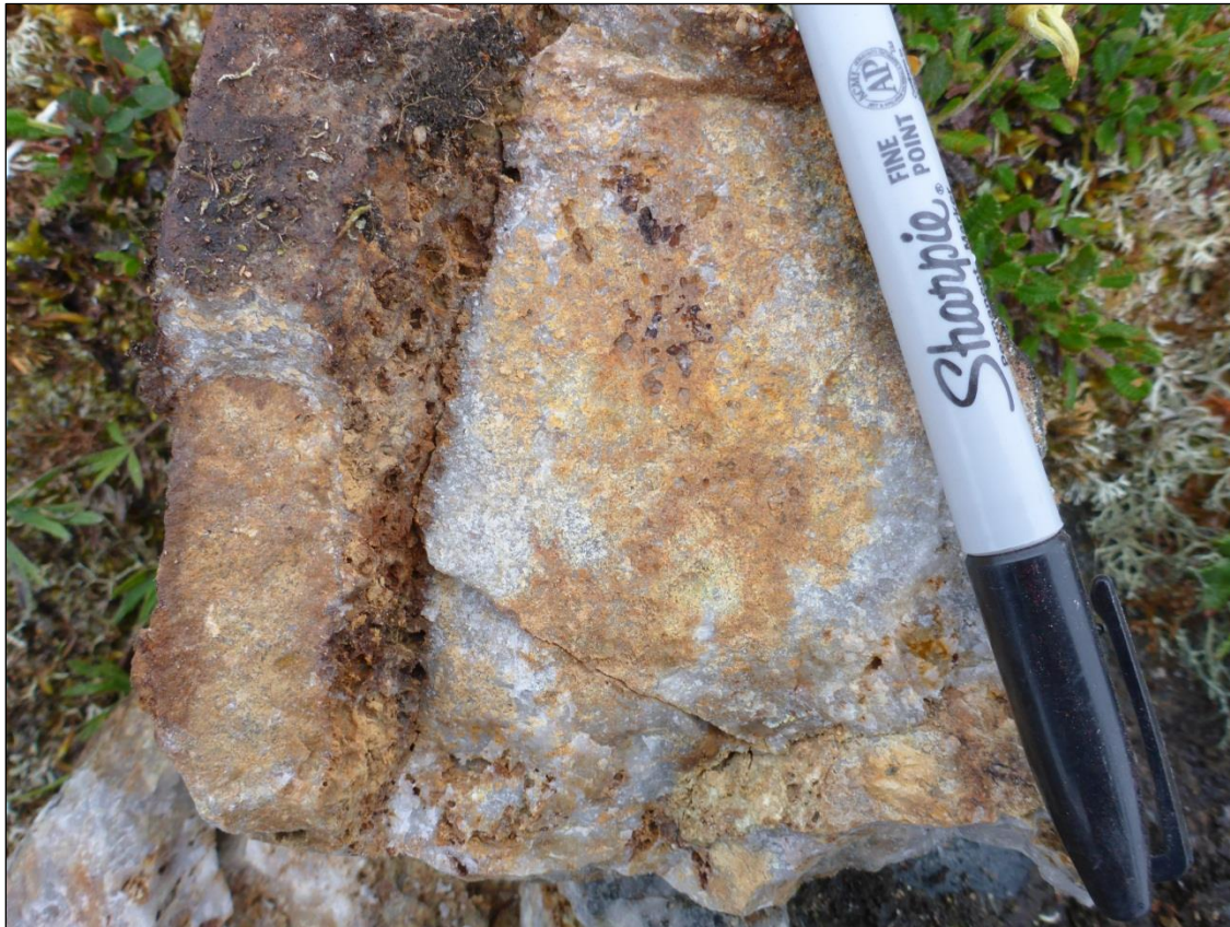
Figure 7: Subcrop grab sample of vuggy quartz vein with limonite boxwork; sample returned anomalous silver, lead and gold assay values (YTG_2013_ECL_0025).
