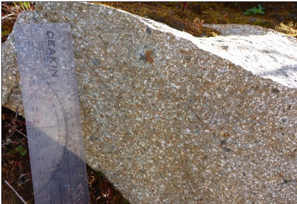
Figure 5: Relatively unaltered, 'crowded' feldspar porphyry with fine-grained, mafic groundmass and trace disseminated pyrite (YTG_2013_ARB_0127).
