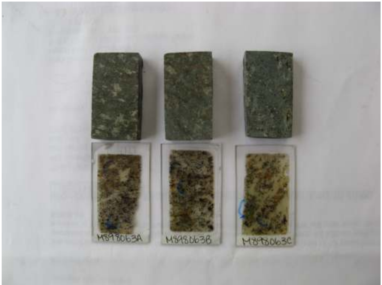
Overviews of thin sections and offcuts (blue semi-circles mark photomicrograph locations).
