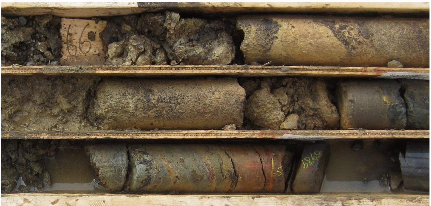
Plate 8: Extremely weathered diorite above the contact with silicified quartzite (at 68.6 m). The diorite contains brecciated sections with Mn-oxide stained and limonitic fragments. The diorite has been altered to clay in situ. Drill hole HLD13-13, 66-68.6 metres.
