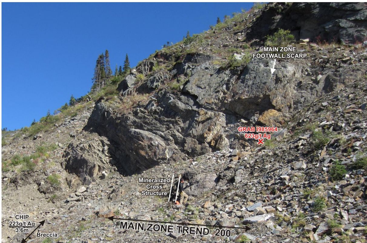
Plate 2: Main Zone, looking across zone to east. Outcrops in background are in the footwall to zone and central outcrop contains a mineralized pyrolusite-rich breccia striking roughly perpendicular to the main trend (200°). Chip sample from outcrop in lower left corner returned 223 g/t Ag over 3.6 metres.
