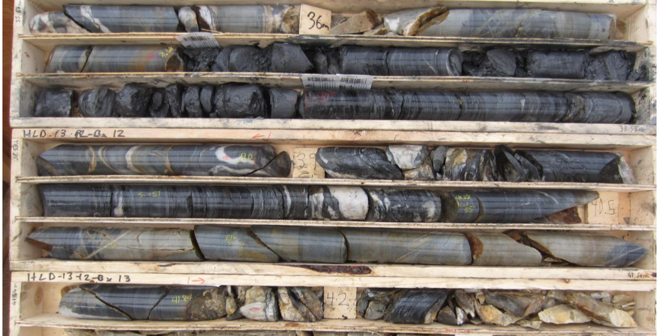
Plate 5: Dark coloured, weakly carbonaceous phyllite, from about 37-40 metres, interbedded with quartzite (drill hole HLD13-12, 36-42 metres).
