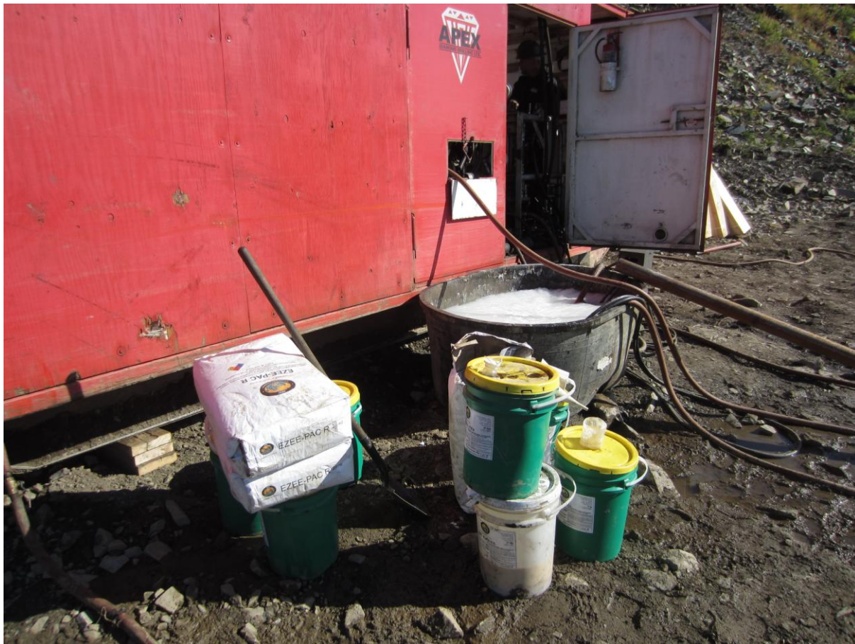
Plate 1: Different types of drill mud used in combination as a part of the 2013 drilling mud program that was intended to assist in recovery of friable core, which is characteristic of the mineralized zones at the Haldane project.
