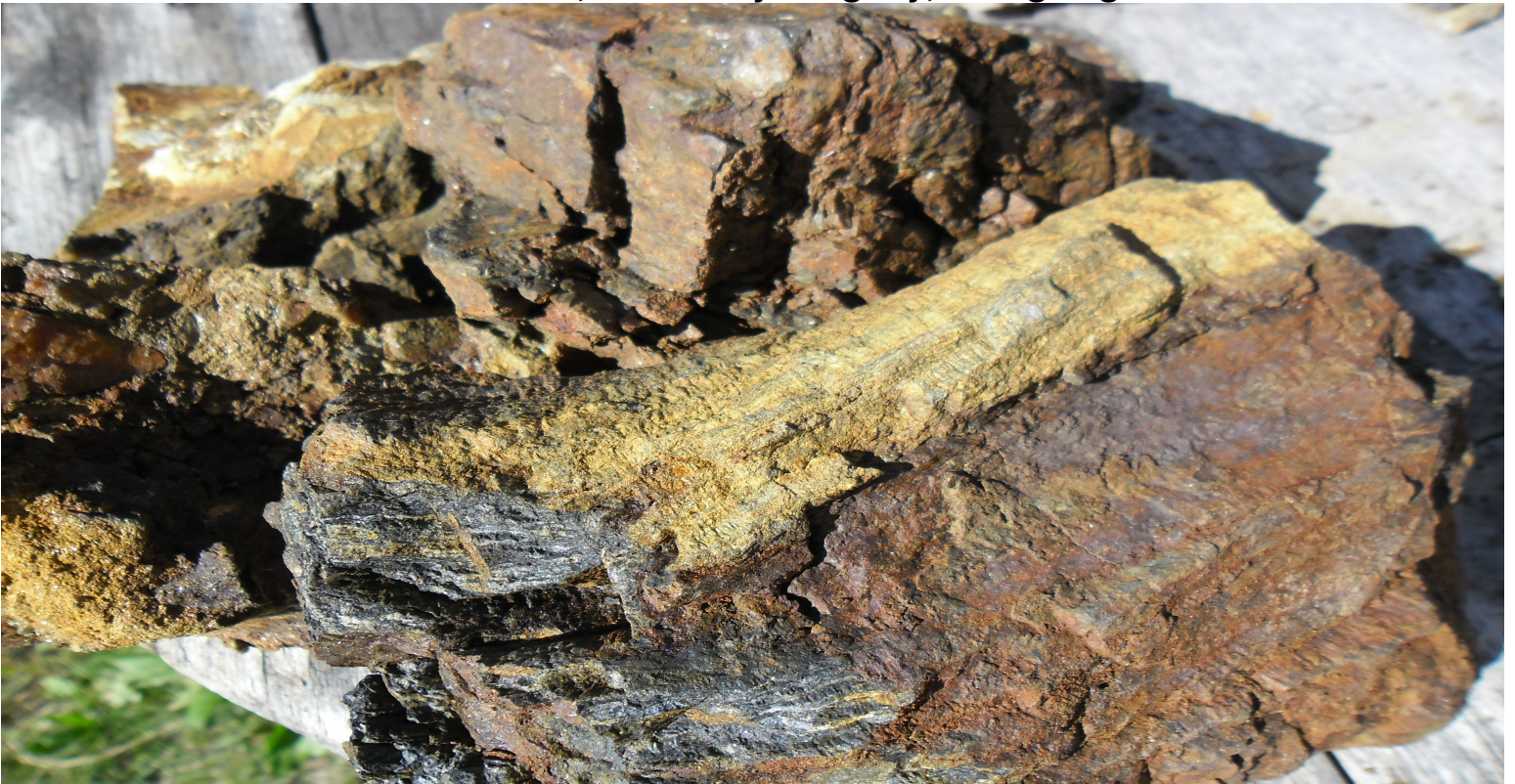
Crushed, pulverized and oscillated with a professional & objective observers witnessing. Erini Petroutsas & Don Kenzie. Gold recovered from this rock type has a coarse texture. Utm Location ~ 07V 596250/7096431 – (W4PulvAu)
