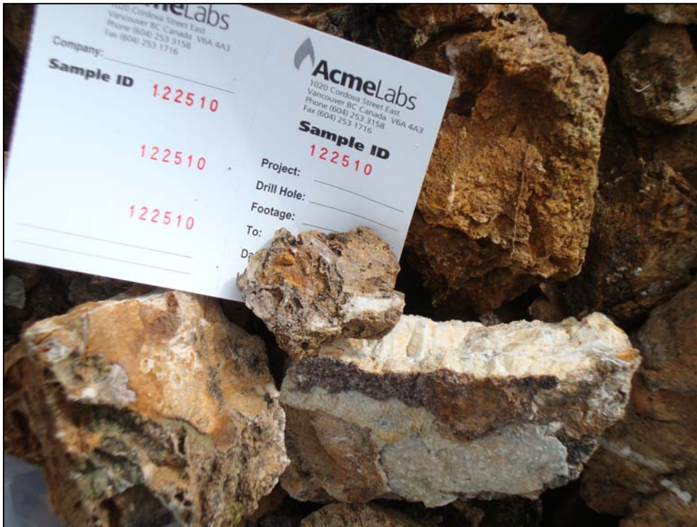
West Zone. Rock float sample 122510; 101 ppm Au, 1004 ppm As, 121 ppm Sb, calcite veins cutting listwanite.
