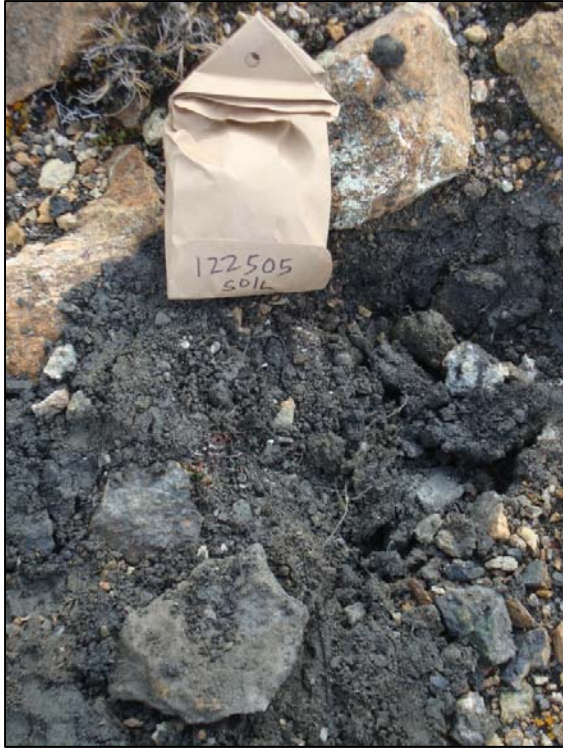
North Zone. Soil sample 122505, 16.5 ppb Au, 680.3 ppm As, 35.27 ppm Sb, grey graphitic 'soil' and listwanite float.
